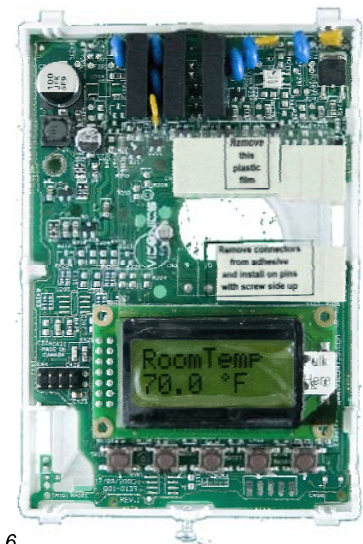
Thermostat assembly (VT7300F1000 shown)
